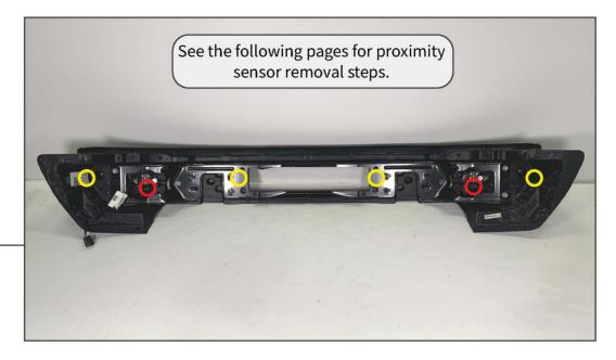
Unplug the wiring harness from each fog light and proximity sensor, if applicable. The proximity sensors can be used on the new bumper.
