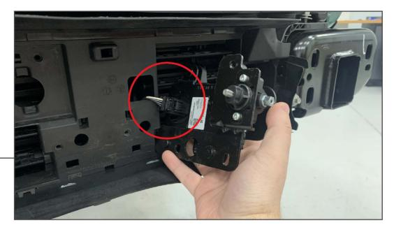
Unplug the ACC module from the shutter assembly wiring harness.
