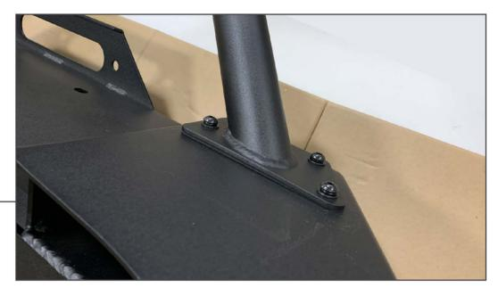
Secure the over rider bar to the bumper using (6) M8 x 25mm Allen bolts, (6) M8 flat washers, and (6) M8 flange nuts. Tighten until secure.
