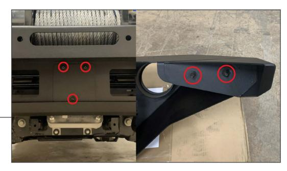
Install the bumper end caps using (2) M6 x 30mm bolts, (4) M6 flat washers, (2) M6 lock washers, and (2) M6 nuts per side. Install the Adaptive Cruise Control (ACC) block off plate OR the vehicle ACC module to the bumper using (3) M6 x 30mm bolts, (6) M6 flat washers, (3) M6 lock washers, and (3) M6 nuts.
