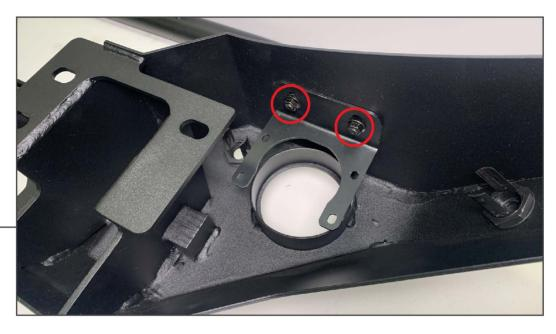
Secure the fog light bracket to the bumper using (2) M8 x 25mm Allen bolts, (2) M8 flat washers, and (2) M8 flange nuts. Ensure the hardware passes through the over-rider bar, bumper, and fog light bracket.
