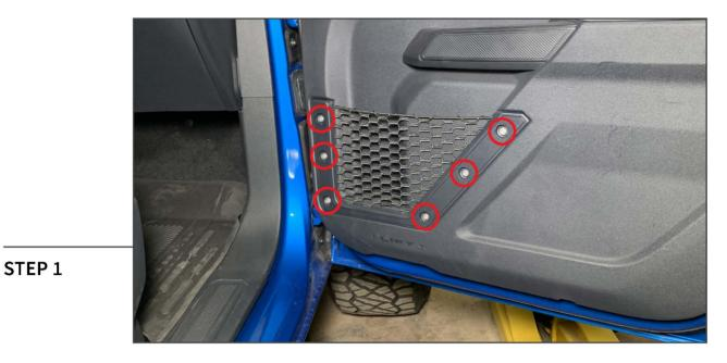
Remove (6) T-30 Torx bolts from the door panel. Do not remove the door panel netting.
