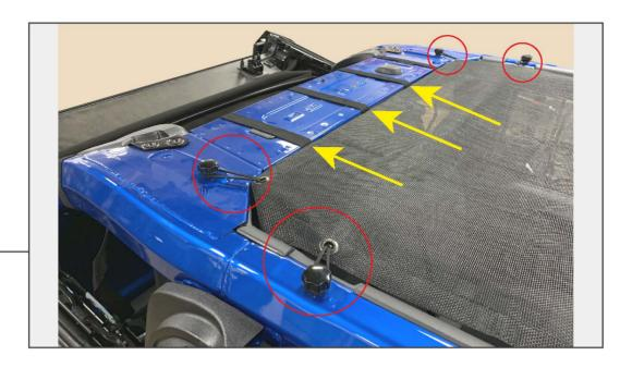
Install (4) thumb screws into the threaded holes in the vehicle roll bar. Once fully threaded in, secure the rear corners of the sun shade using (4) elastic bands.
