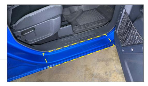
Using the designated door entry guard, test fit the guard to the vehicle before removing the adhesive tape.
