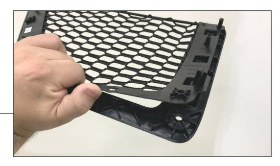
Separate the netting layer from the vehicle panel.
