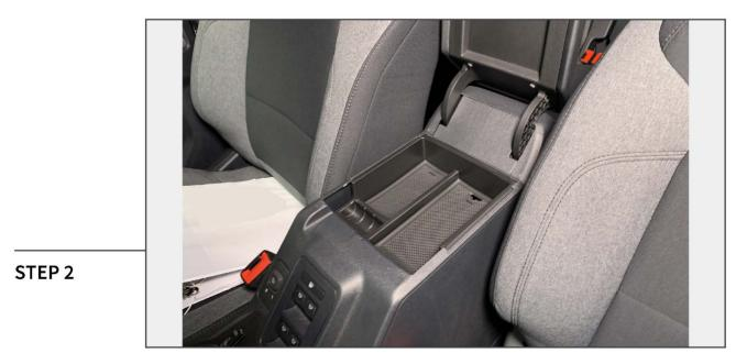
Place the storage tray into the center console. The tray will fit within the outer edges of the center console.
