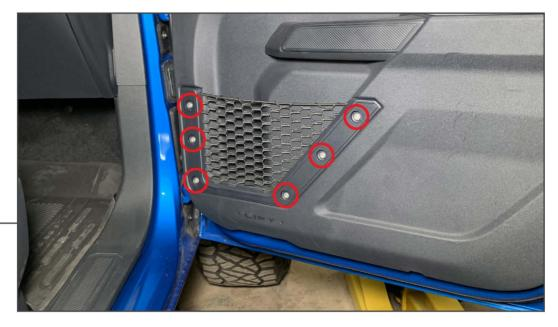
Remove (6) T-30 Torx bolts from the door panel. Do not remove the door panel netting.
