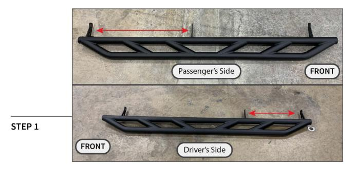
Lay out the rock sliders, and identify each side. Take note to the spacing of the center to rear mounts.
