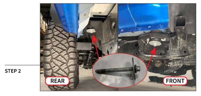
Remove the (1) center 15mm body mount bolt from each body mount.
