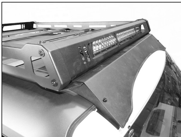
(Fig 27) LED bar style light installed (driver/left side pictured-light not included)
