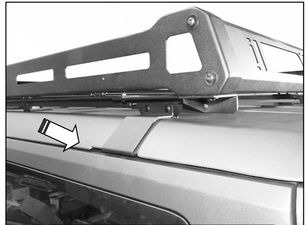
(Fig 21) Hook Clamping Bracket into slot in of top above window
