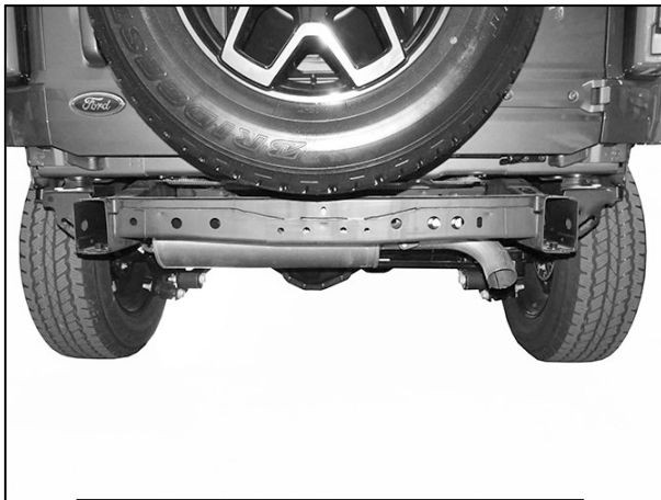
(Fig 3) Remove bumper assembly
