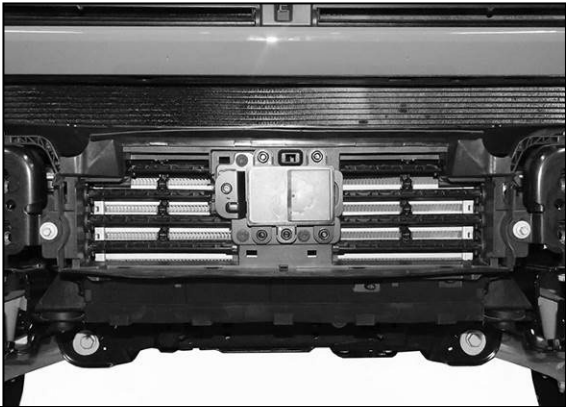
(Fig 5) Remove the shutter assembly. Models with ACC sensor (pictured), unplug and remove sensor from shutter assembly
