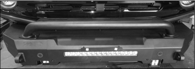
(Fig 32) Reinstall center Cover Plate
