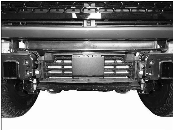
(Fig 4) Remove factory hex bolts from front to remove bumper assembly
