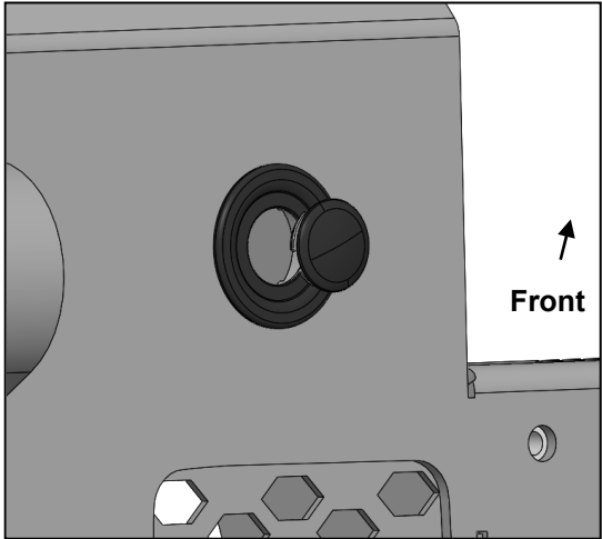
(Fig 18) Models without parking sensors, push the included Plugs into sensor mounts
