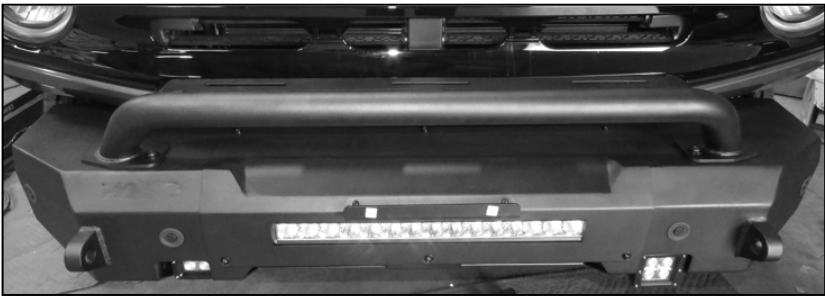
(Fig 32) Reinstall center Cover Plate
