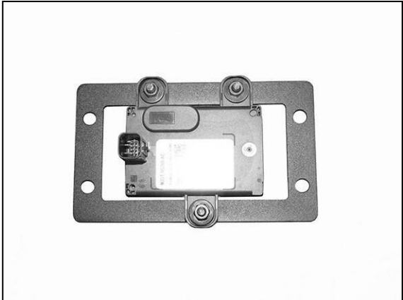
(Fig 15) ACC sensor attached to Bracket
