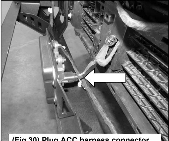
(Fig 30) Plug ACC harness connector into ACC sensor
