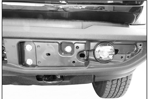
(Fig 2) Models with plastic bumper cover (see Fig 1), remove bumper pads from bumper (driver/left side pictured)
