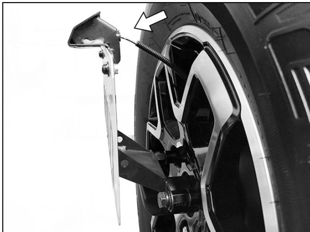
(Fig 20) Plug Harness into license plate light
