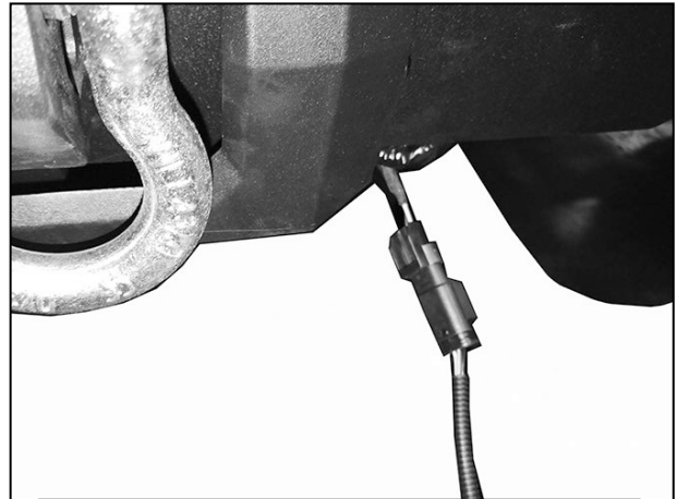
(Fig 15) Plug the long License Plate Light Harness into the factory wiring harness on the Bumper for the license plate light
