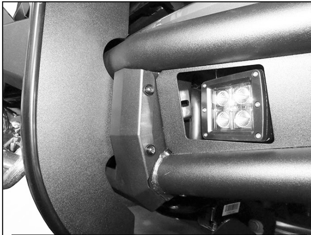
(Fig 7) After Push Bar is aligned and all hardware fully tightened, reinstall U-Covers
