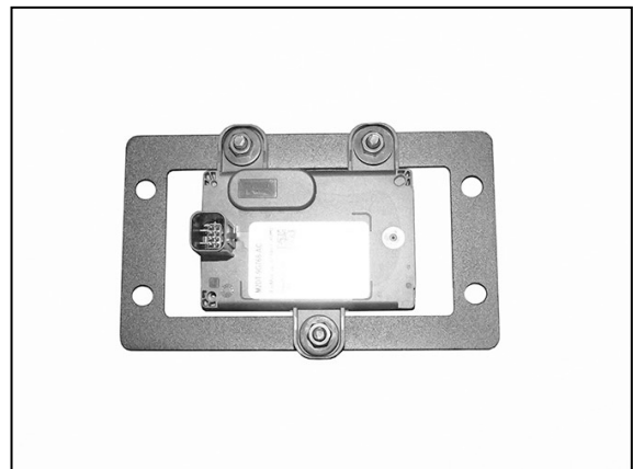
(Fig 13) ACC sensor attached to Bracket
