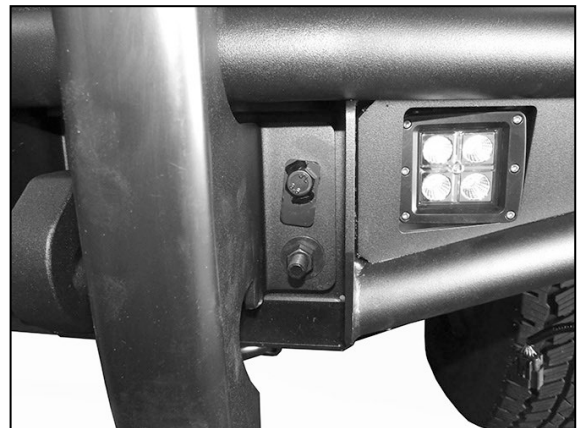
(Fig 6) Driver/left side of Push Bar attached to Bumper
