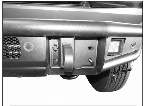
(Fig 4) Offset Shack Mount installed
