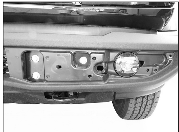
(Fig 2) Models with plastic bumper cover (see Fig 1), remove bumper pads from bumper (driver/left side pictured)
