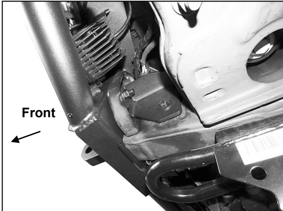
(Fig 27) Driver/left side of Bumper attached to outer Single Bolt Plate pictured from below
