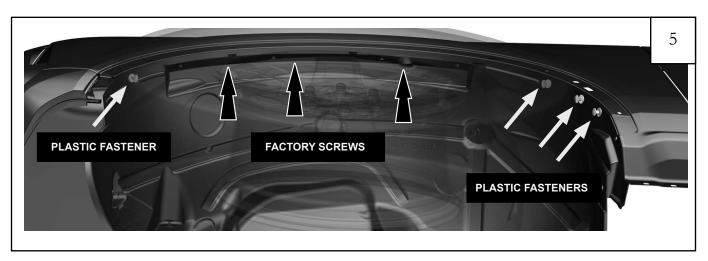
Remove (4) factory plastic fasteners and (3) factory screws to access backside of fender.
