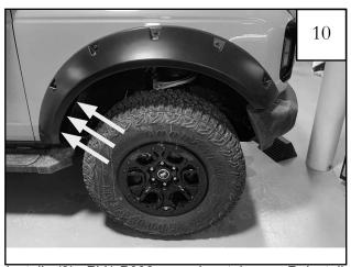
Install (3) RV1-P008 panel retainers. Reinstall factory fasteners removed in **Step 5**. Front flare installation complete.
