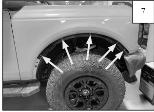
Install inner bracket using (5) SW1-0008 bolts, (10) WA1-0015 washers, and (5) NU1-0016 nuts. (See diagram Step 8)
