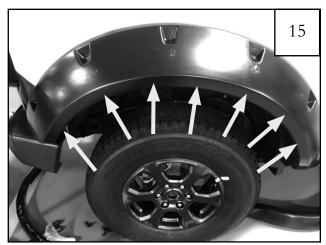
**NOTE:** Ensure that edge trim is seated correctly before proceeding. Press flares firmly onto the vehicle and install and fully tighten (8) SW1-0058 screws.
