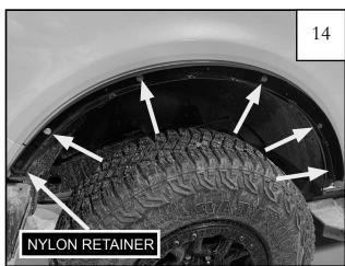
Install inner bracket Using (5) factory body bolts, and (1) RV1-P006 nylon retainer.
