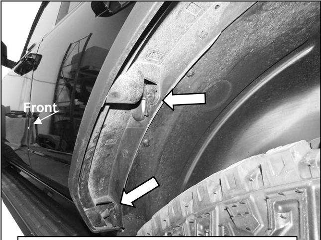
(Fig 1) Locate the clips under the factory fender, turn the clips counter clockwise. Carefully pry the fender away from vehicle
