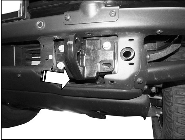
(Fig 5) Models with steel bumper, insert Upper Bracket between tow hook and opening in bumper (arrow). Attach end of Bracket to bottom of frame, between frame and splash guard bracket. Reinstall splash guard/skid plate and cover
