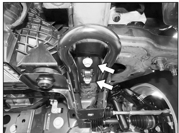
(Fig 2) Remove plastic cover surrounding tow hook. Loosen tow hook bolts (arrows)
