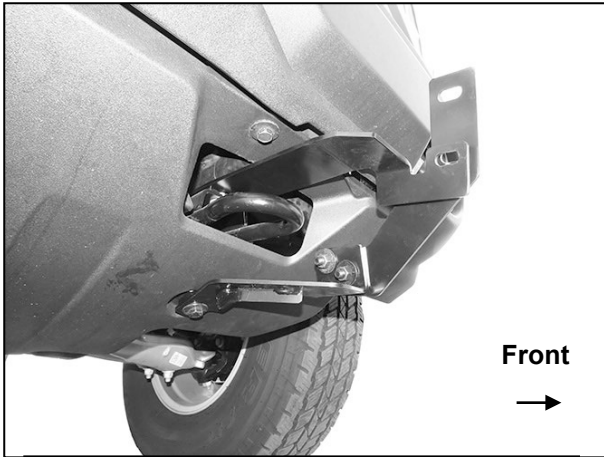
(Fig 11) Driver/left side Brackets installed
