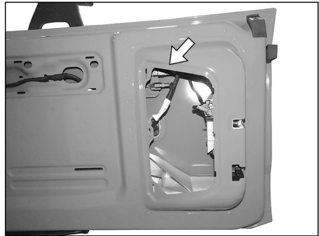
(Fig 2) Disconnect wire harnesses leading to the camera and CHMSL (3rd brake light). Release rubber grommet and pull harness through hole in rear door
