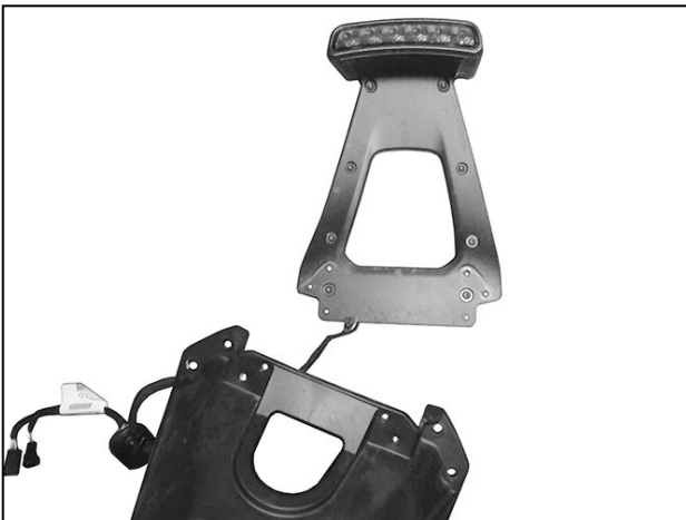
(Fig 6) Remove the brake light assembly from the top of the spare tire mount
