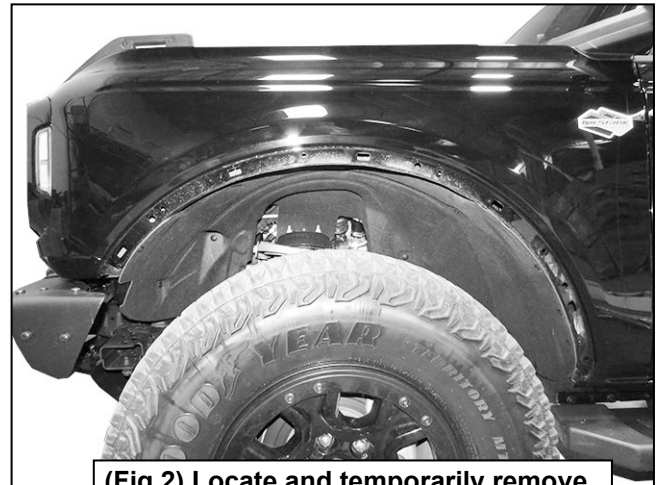
(Fig 2) Locate and temporarily remove the hardware attaching the fender liner to the edge of the wheel well
