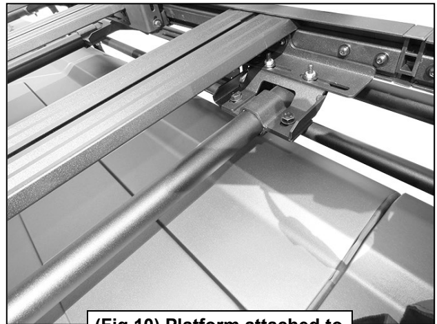
(Fig 10) Platform attached to the crossbars on the vehicle
