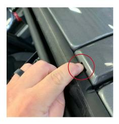
1. Press the tab on the accessory ready mount cover on the topside of the windshield frame using a plastic trim removal tool or your finger tip and remove the cover. 4. Repeat steps 1 through 3 on the other side of the vehicle.
