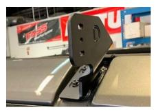
3. Using the nuts removed in step 2, install your new windshield bracket as shown in the picture to the left. Photo is showing the driver side of vehicle. Note that the DD logo is facing out.
