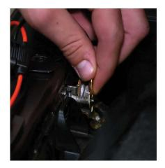
8. Connect positive and negative battery wires to the battery, or to main power terminals near the fuse box.
