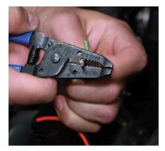
7. Locate the auxiliary switch wiring in the engine bay. Access the owner's manual in the head unit to determine which wires you'd like to use. Since this harness draws main power directly from the battery, you can use any wire to supply a power signal to the SS5 main beam as well as the backlight. Using wire strippers, remove enough insulation to make a good connection. Insert the wire into the butt connector and crimp it to secure the connection.
