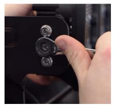
6. Then install the assembled SS5 lightbar on to the brackets with provided the M6 flange screws. Adjust supports as needed.
