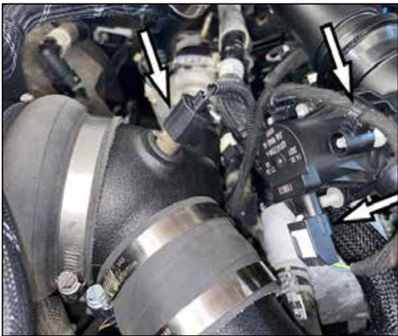
25. Reconnect the IAT sensor and BOV electrical connections and secure the BOV harness to the stud.
