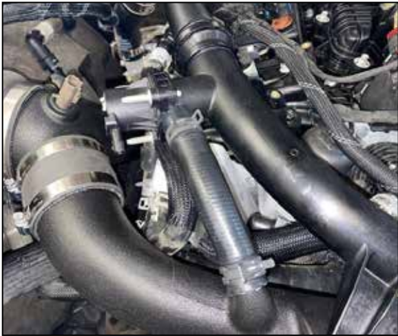
24. Install the BOV hose onto the fitting on the K&N intake tube and secure with the provided spring clamp.
