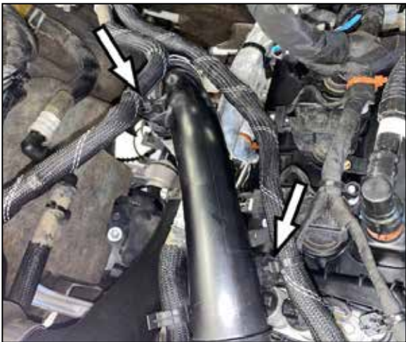
26. Resecure the coolant hoses to the hot-side charge tube.
