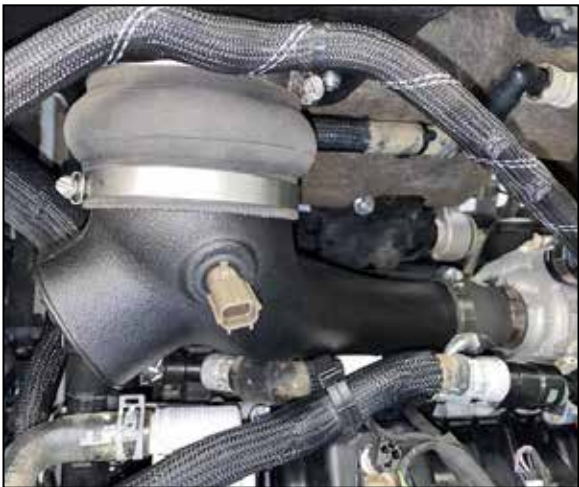
18. Install the K&N intake tube into the coupler at the turbo inlet and then into the coupler at the filter adapter and secure with the provided hose clamps.
