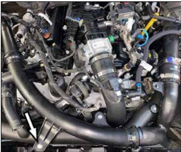
22. Reinstall the factory hot-side charge tube and secure the three connections. Reinstall the factory mounting bolt that secures the tube to the core support.
