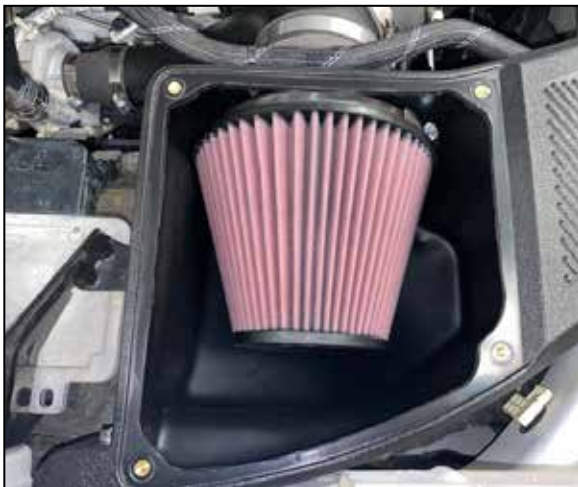
27. Install the K&N air filter onto the filter adapter and secure with the provided hose clamp.
