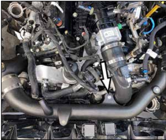
20. Install the driver side K&N intake tube into the factory turbo inlet coupler and then into the coupler on the passenger side K&N intake tube, adjust the tube for best fit and secure with the hose clamps and bolt.
