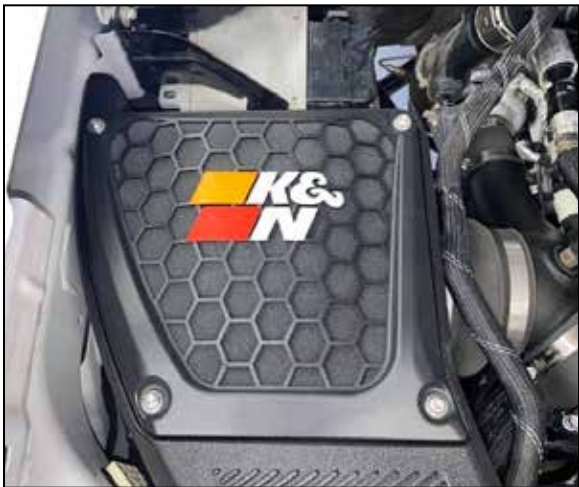
28. Assemble the filter top and then install the assembly on top of the air filter housing and secure with the provided hardware.
