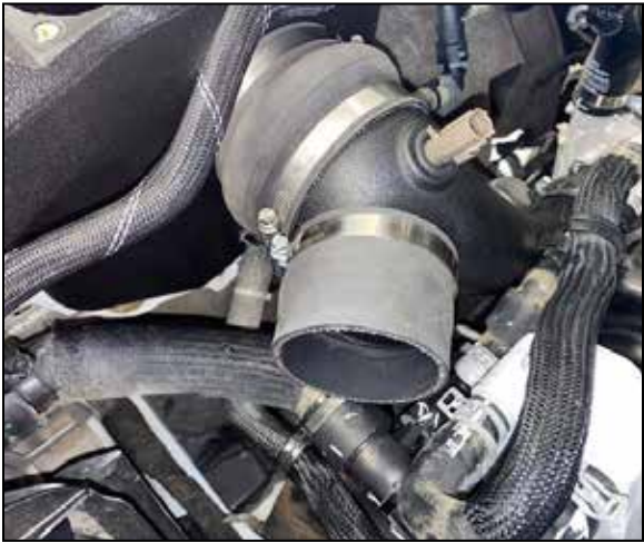
19. Install the remaining straight coupler onto the K&N intake tube and secure with the provided hose clamp.
