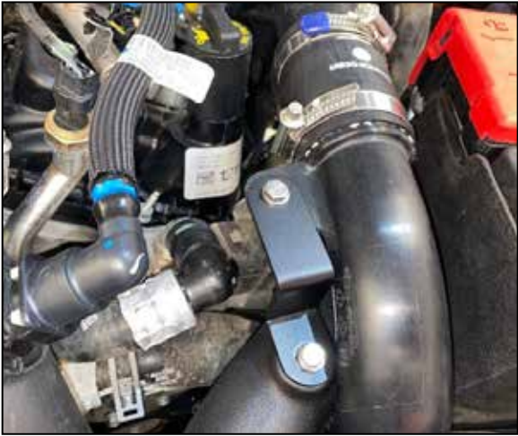
23. Install the provided "Z" bracket to the hot-side charge tube and K&N driver side intake tube and secure with the provided hardware.
