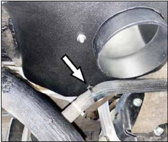
15. Secure the lower coolant hose to the air filter housing.
