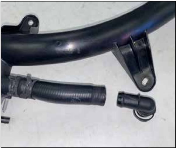
21. Release the spring clamp that secures the quick connect fitting onto the BOV hose and then remove the fitting from the hose.
