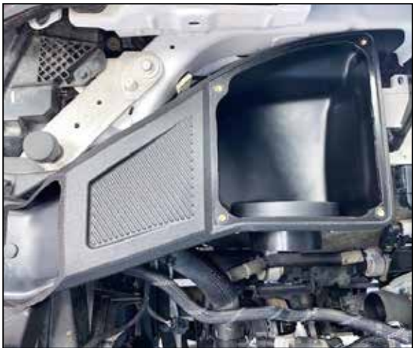
14. Set the K&N air filter housing into position and secure with the factory push-pin and the provided bolt.
