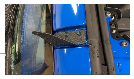
Install the designated light bar mounting bracket to the vehicle using the (2) original 10mm nuts. Do not fully tighten nuts to allow for adjustments later.
