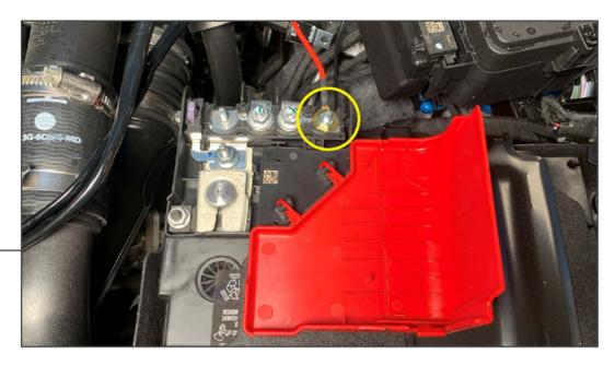
Secure the positive lead to the unused battery stud using the included (1) M6 flange nut.
