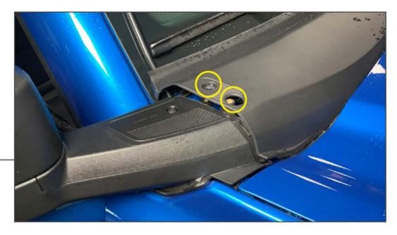
Plug the light bar into the included light bar wiring harness. Tightly secure the wiring harness down the side of the windshield using the (4) adhesive cable mounts. Remove (1) T-30 Torx bolt from the windshield cowl, and remove the antenna using an adjustable wrench. Tuck the wiring harness into the cowl, then re-install the (1) T-30 Torx bolt and the antenna into the vehicle.
