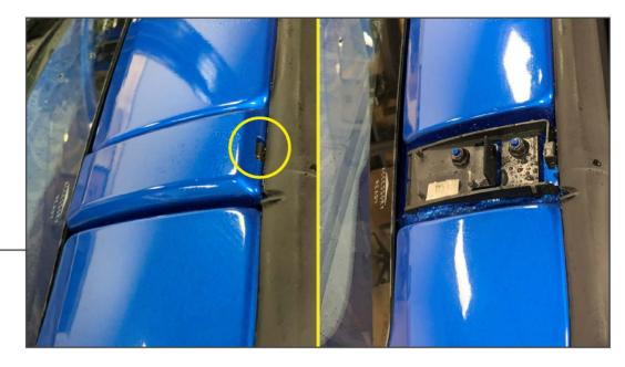
Locate the accessory mounting point above the windshield on each side of the vehicle. Press the plastic tab inwards to release the painted cap from the vehicle.
