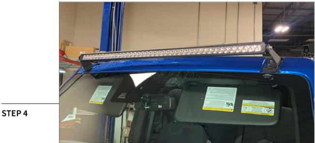
Mount the light bar to the brackets using (2) M8 x 15mm Allen bolts, (2) M8 lock washers, and (2) M8 flat washers. Tighten the hardware evenly. Ensure light bar harness is on the RH side of the vehicle when installed.
