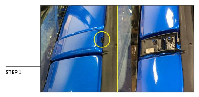
Locate the accessory mounting point above the windshield on each side of the vehicle. Press the plastic tab inwards to release the painted cap from the vehicle.
