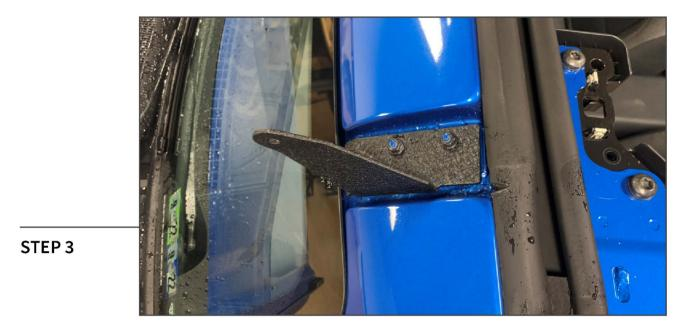
Install the designated light bar mounting bracket to the vehicle using the (2) original 10mm nuts. Do not fully tighten nuts to allow for adjustments later.
