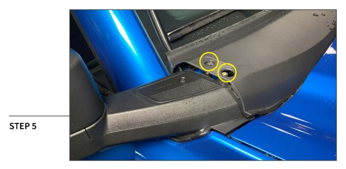
Plug the light bar into the included light bar wiring harness. Tightly secure the wiring harness down the side of the windshield using the (4) adhesive cable mounts. Remove (1) T-30 Torx bolt from the windshield cowl, and remove the antenna using an adjustable wrench. Tuck the wiring harness into the cowl, then re-install the (1) T-30 Torx bolt and the antenna into the vehicle.
