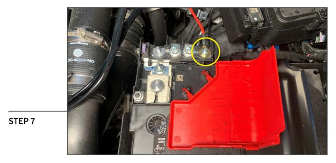
Secure the positive lead to the unused battery stud using the included (1) M6 flange nut.
