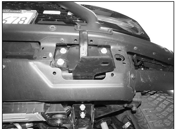
(Fig 6) Models with steel bumper, insert Support Bracket between tow hook and opening in bumper. Attach end of Bracket to bottom of frame and splash guard bracket
