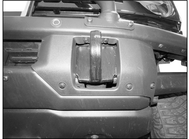
(Fig 4) Model with steel bumper, remove cover from bumper (driver/left side pictured)
