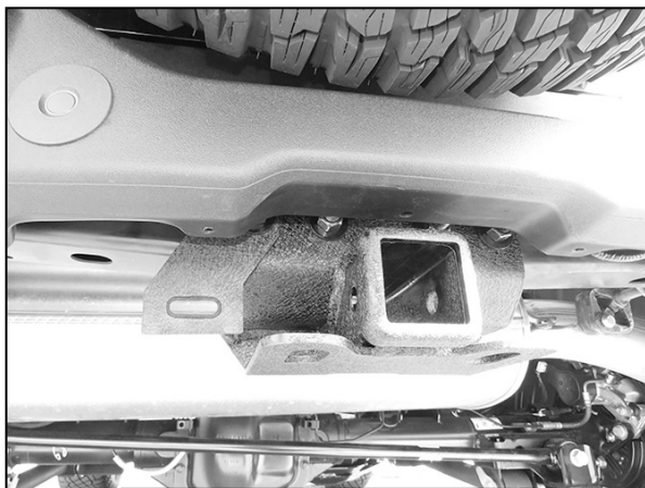
(Fig 5) Receiver Hitch and Harness Bracket installed
