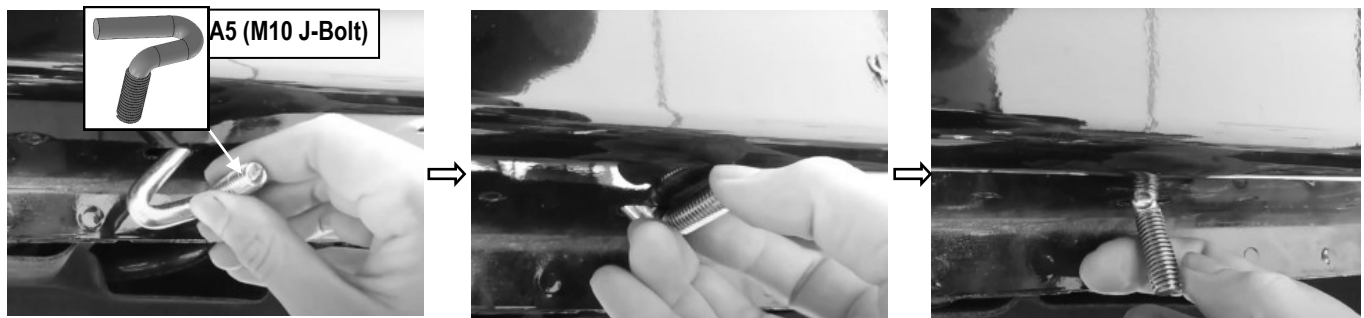
(Fig 6) A5 (M10 J-Bolt) Installation (On Driver Side Mounting Location)
