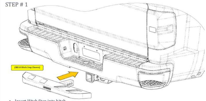
· Insert Hitch Step into hitch.
